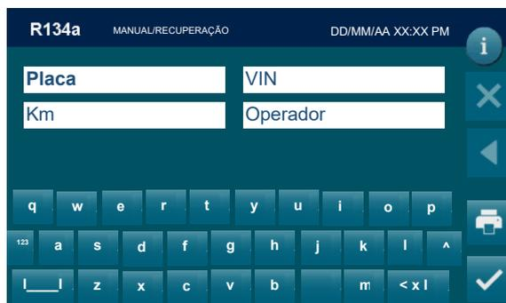
Introduza a matrícula do automóvel, VIN, Km, Operador e prima
