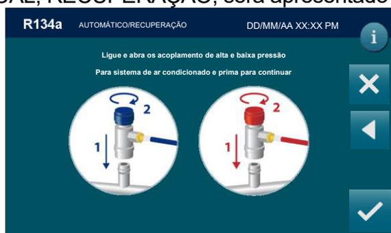
Ligar e abrir o acoplamento ao sistema de ar condicionado, em seguida, prima
